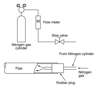
Fig. 3-5-1 Prevention of oxidation during brazing
