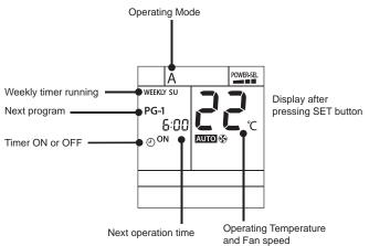
\*Point remote control at air conditioner receiving module then, press SET button until you hear the "PiPi" sound. This means the setting operation has been completed.
