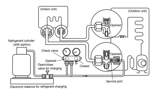
Fig. 3-4-1 Configuration of refrigerant charging
