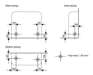
1. After determining the pipe hole position, drill the pipe hole ( $\varnothing$ 65 mm) at a slight downward slant to the outdoor side.
