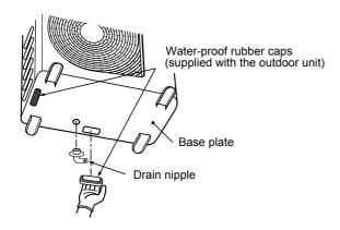
2. Install the drain nipple and a commercially available drain hose (with 16 mm inside diameter), and drain off the water.
